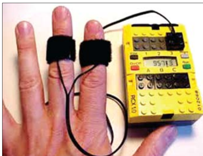
FIG 1: Galvanic Skin Response Instrument for Monitoring Stress
